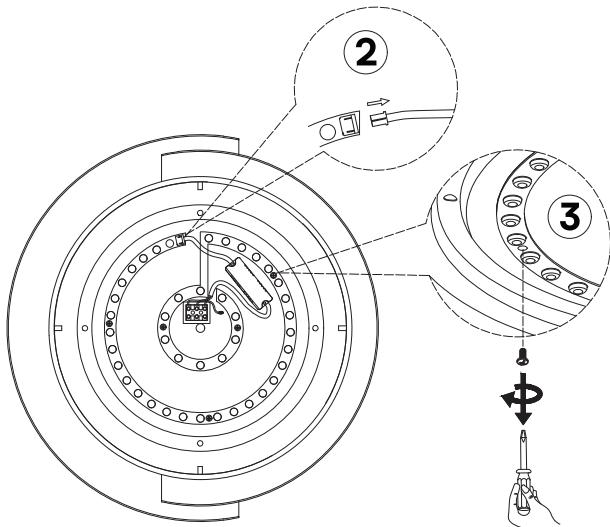
2. Remove the SM terminals on the driver and LED strip.
