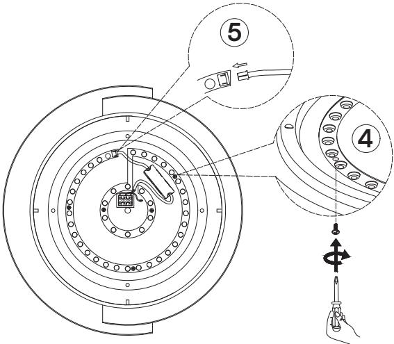
4. Install a new LED strip and secure it with screws.
